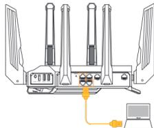
[Wireless] Connect to the network with default SSID shown on the product label on the back side of your router "ASUS\_XX".
